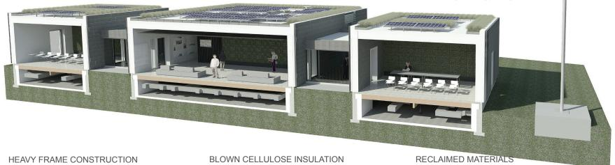
The structural frame of Galileo's Pavilion is over three times as thick as conventional framing which allows more insulation to be used between the structural components. Engineered lumber, a product project it is used with engineered lumber to create that maximizes wood's potential, is used throughout the frame construction. All of the construction joints are caulked or foamed and the entire assembly is pressure tested (a blower door test) to assure its tightness.
